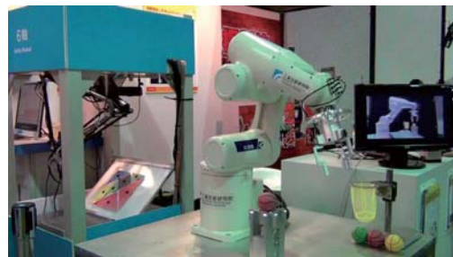
Teaching robot by lead through
