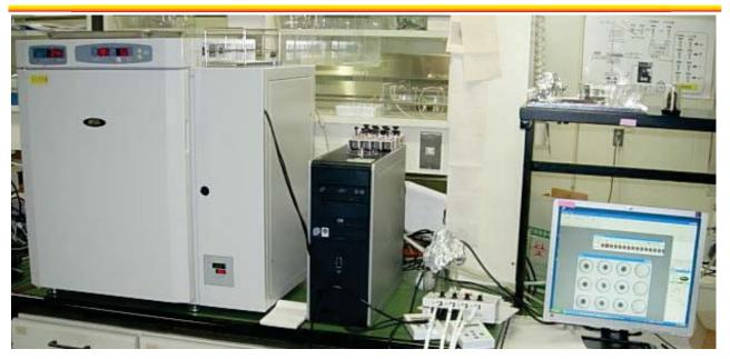
Real-time culture cell monitoring system (Astec, Fukuoka, Japan)
